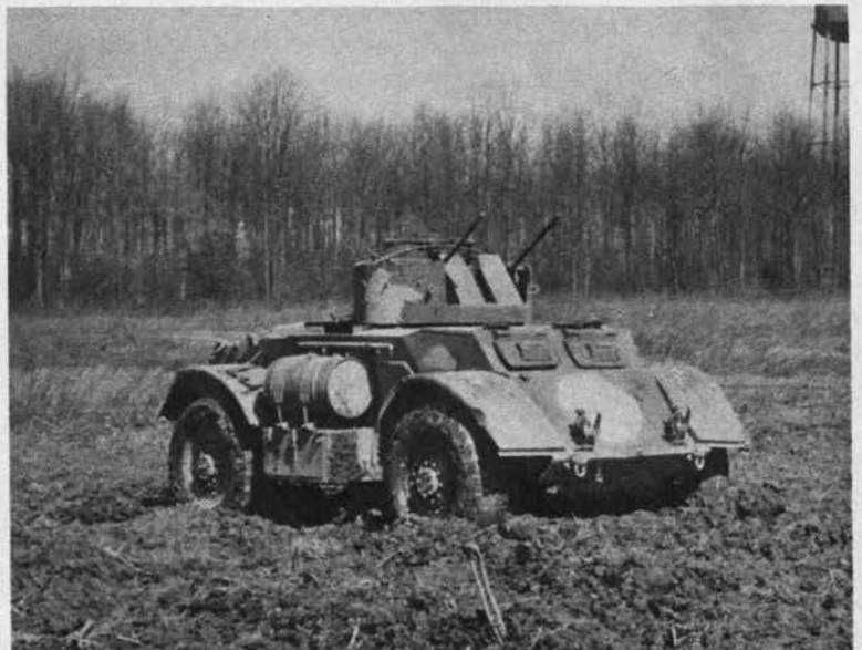
T-17E2 is the anti-aircraft version of the T-17E1 at the left. A special circular, open-topped turret carries twin AA guns. U. S.-built, the T-17E1 and T-17E2 have wide round fenders, jettison tanks at sides.
